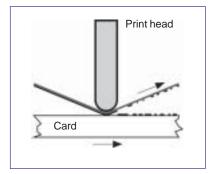
The K (black) panel is a resin that "mass transfers" onto the surface of the card, instead of migrating into it. With mass transfer the printer has little control over a pixel's size or density - it's either there or it isn't. K printing is used for bar codes because it is machine readable, whereas YMC dyes are not.
