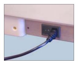
Power cord entry and ON-OFF switch are located on the rear panel.
