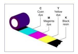
This is the usual pattern for a P640i Printer ribbon. Y, M and C are the three "dye sub" process colors. The K panel is for infrared-readable bar codes and other data, usually on the back of the card. A second K panel (YMCKK) is sometimes provided to allow black resin printing on both sides of the card.
