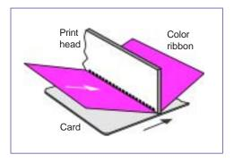
As the ID card is driven through the print station, the color ribbon is metered out from the supply roll at the same speed. Each color regires a separate "pass" of the card. The black dots at the bottom edge of the print head depict the heating elements - in practice, at 300 to the inch, they are too small to be seen with the naked eye.
