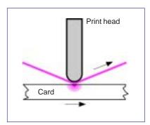
Color migrates from the dye ribbon onto the ID card, the spread of the dye depending on the amount of heat applied by the print head element. Each time it comes to a dye panel boundary, the print head lifts to allow the card to back up, then lowers again to print the next color.
