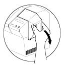
**1** • Open Card Feeder Cover by putting your fingers on both sides and rotating the cover in a clockwise direction to the open position.
