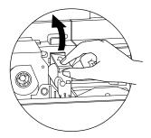
**2** • Gently remove Cleaning Cartridge by rotating up and away from printer.
