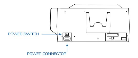
Place the printer's power switch in the OFF (  ${\rm O}$  ) position.
