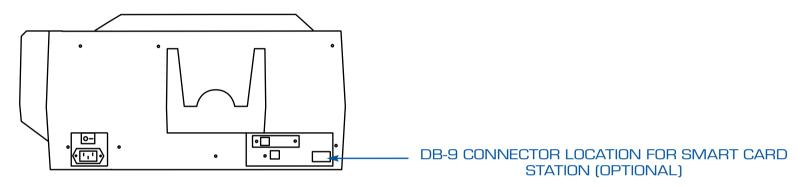
An attached external smart card programmer can be used to program smart card chips. The following table shows the smart card contact points.
