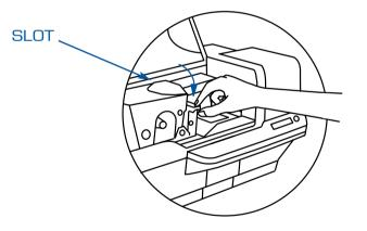
4 Hold the card cleaning cartridge by the extended 'handle' (so the large arrow on the top is pointing away from you). With the cartridge at about a 30° angle (pointing downward), insert the lip of the cartridge into the slot, until the cartridge seats against the back wall.
