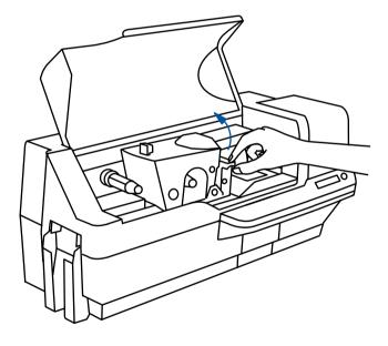
3 Remove the cleaning roller from the card cleaning cartridge and discard.
