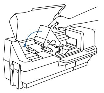
**Note:** During normal operation (with power connected and turned on), the ribbon would automatically synchronise when the printhead is restored to its fully-down position. The ribbon would be identified and the corresponding parameters sent to the driver.
