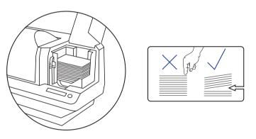
Open card feeder cover and place the cards in the input hopper.
