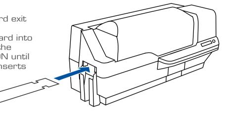
**Note:** If the user does nothing at this point (ie., does not insert the long cleaning card), after a timeout the LCD panel display will change to CLEAN PRINTER. The printer will be able to print, but the LCD panel will continue to display CLEAN PRINTER.
