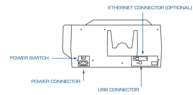
If your printer includes the optional Ethernet Adapter as well as the standard USB connection, use either the supplied USB cable or a standard Ethernet cable to connect the printer to a corresponding port on the computer or network.
