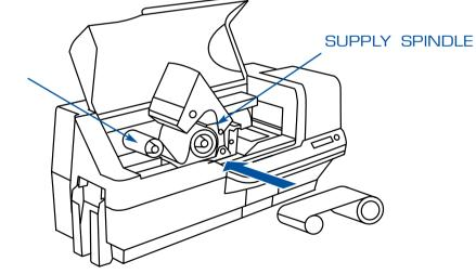
3 Locate the ribbon supply spindle and the ribbon take-up spindle (see above). Load ribbon onto the supply spindle (under the printhead carriage) flange side in, and load the empty core (with tape attached) onto the take-up spindle. Make sure the ribbon comes off the top of the supply spindle and feeds to the top of the take-up spindle. 4 Gently press the printhead carriage down until it is fully lowered, as shown below. Very little force is necessary to perform this step.
