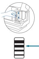
This item can be operated by the user to set the card thickness and to prevent more than one card feeding into the printer at the same time and causing a jam.
