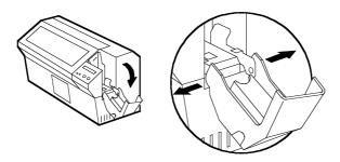
A. Open card cartridge cover B. Carefully release cover pivots from printer Store card cartridge cover for possible later use.
