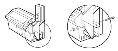
Position stacker INSIDE the metal arms. Feed long bolt through the holes. Add washer and apply wing nut. Do not over-tighten.
