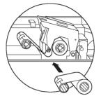
**3.** Load ribbon onto the supply spindle (under print head carriage) and empty core (with tape attached) onto the take-up spindle. Make sure the ribbon comes off the top of the supply spindle and feeds to the top of the take-up spindle.
