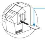
2. Remove any normal cards from the card cartridge. Insert one pre-saturated cleaning card (provided) through slot on the rear of the card cartridge. Close the print head bracket. Close the cover.
