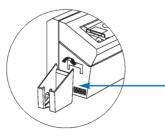
Install card output hopper to printer by hooking over bottom edge of card exit aperture.
