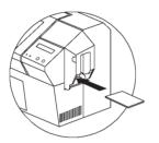
For one-at-a-time printing, feed cards through slot on rear of card cartridge.
