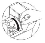
Open cover, and adjust lever to the correct position for the card thickness you are using. Repeat for different card thickness. (Factory setting is for 30mil (0.762 mm) card thickness). See diagram below :
