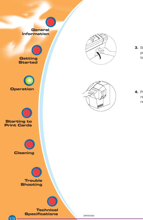
**3.** Swing up the reject card box door and press the top. An audible "click" signals the locked position.
