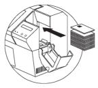
Position the cards with the smart card chip at the top of the card and towards the printer.
