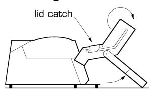
Lift stacker legs off base and rotate stacker back.
