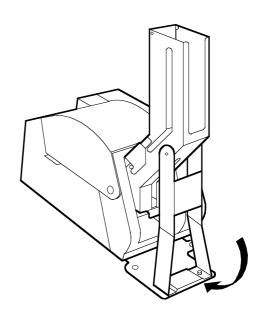
2. Rotate stacker leg and position over studs on base.
