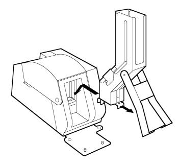
Slide out feeder lock and position stacker onto bar.
