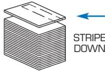
When loading cards into the card cartridge, please ensure that the magnetic stripe is facing down and closest to the rear.
