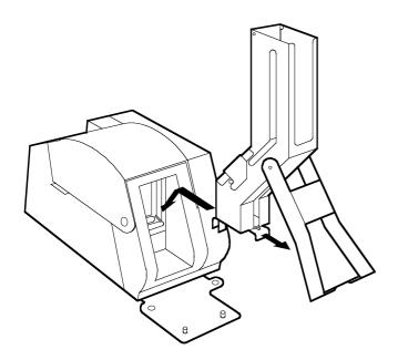
1. Slide out feeder lock and position stacker onto bar. Push feeder lock to secure stacker.
