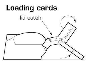
Lift stacker legs off base and rotate stacker back.
