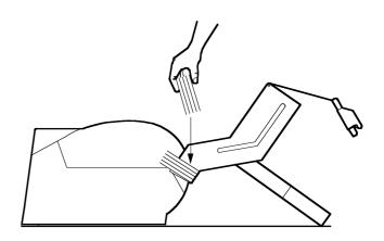
2. Load about 30 cards (only) into bottom of stacker. Ensure cards fall forward, towards printer.
