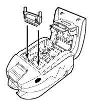
Open lid by pressing the cover release buttons on the sides of your printer. The card cleaning cartridge is packed separately from the printer in a protective plastic bag.
