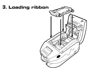
Open lid by pressing the cover release buttons on the sides of your printer. Install ribbon cartridge into the slots and gently press down to engage. Close lid securely.
