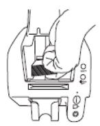
Insert cards as shown. Try only to touch the edges of the card when handling. Make sure cards are laying flat in the J230i hopper.
