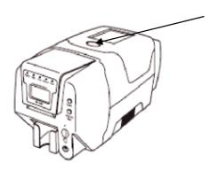
Open the printer lid by pressing the Cover Open button on the top of the printer.
