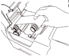
Remove the ribbon from its package and insert as shown. New supply to front, take-up at back. Gears to go to the left.
