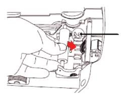
Insert the blue cleaning roller into the U-shaped slots near the front of the printer.
