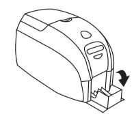
Raise the printer lid and rotate the hopper down.
