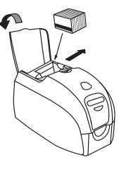
Open card feeder cover. Slide card guide all the way to the right until it locks in place with an audible click.
