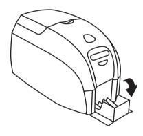
Raise the printer lid and rotate the hopper down.
