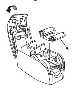
Peel protective wrapper from adhesive cleaning roller by gently pulling on the tape.
