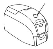
Open printer lid by pressing the cover release button on the top of your printer.
